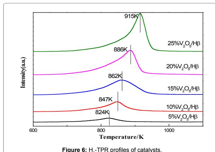
Figure 6: H<sub>2</sub>-TPR profiles of catalysts.
