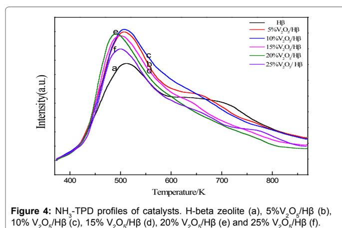
Figure 4: NH<sub>3</sub>-TPD profiles of catalysts. H-beta zeolite (a), 5%V<sub>2</sub>O<sub>5</sub>/Hβ (b), 10% V<sub>2</sub>O<sub>5</sub>/Hβ (c), 15% V<sub>2</sub>O<sub>5</sub>/Hβ (d), 20% V<sub>2</sub>O<sub>5</sub>/Hβ (e) and 25% V<sub>2</sub>O<sub>5</sub>/Hβ (f).
