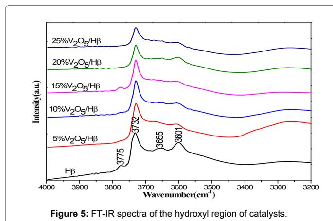
Figure 5: FT-IR spectra of the hydroxyl region of catalysts.
