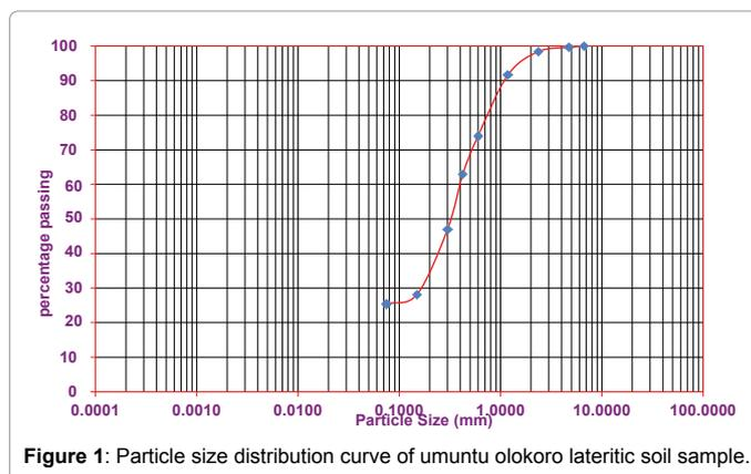
Figure 1: Particle size distribution curve of umuntu olokoro lateritic soil sample.
