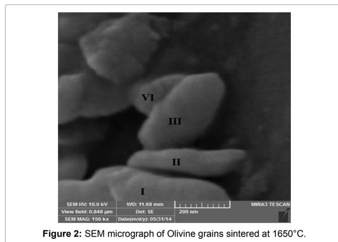
Figure 2: SEM micrograph of Olivine grains sintered at 1650°C.
