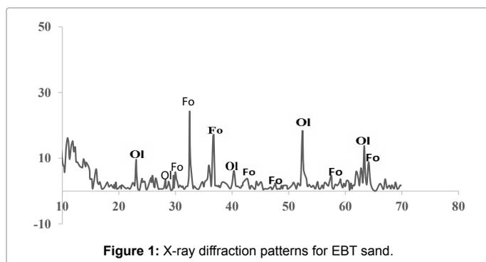
Figure 1: X-ray diffraction patterns for EBT sand.
