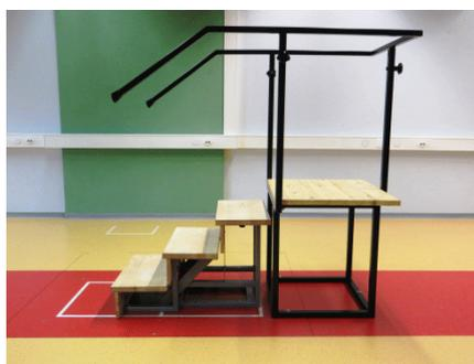
**Figure 1:** Photograph of the stairway set-up on the force plates. The stairway was attached with threaded inserts on the platforms. The stairway allows for measuring isolated forces and moments generated during each of four consecutive steps.
