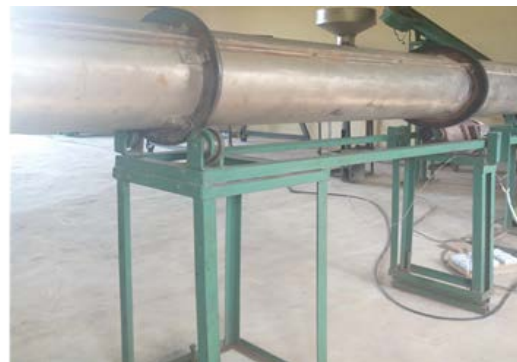
Figure 2: Exterior view of the rotary dryer.
