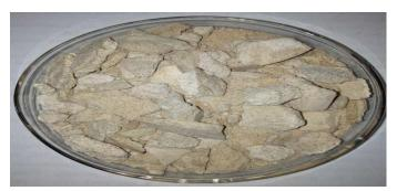
Figure 3: Plate 1: Chitosan obtained after the deacetylation of chitin extracted from shells of water snail, using 40% sodium hydroxide (NaOH) and heating under reflux for six (6) hours at 100°C.
