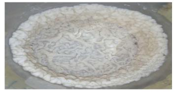
Figure 5: Plate 2: Chitosan hydrogel produced when chitosan was dissolved in 1% acetic acid and concentrated at  $75^{\circ}$ C.
