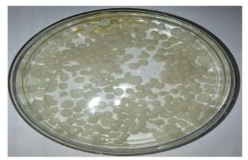
Figure 6: Plate 3: Chitosan beads formed in precipitating colloidal sodium hydroxide solution.
