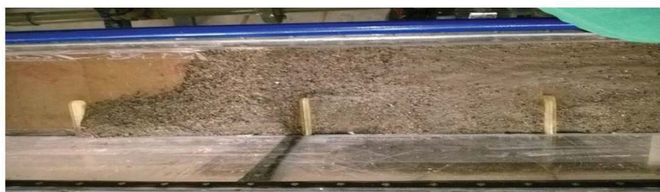
Figure 6: Sand bed after test on Groynes with depth of sand of 1.5 cm.
