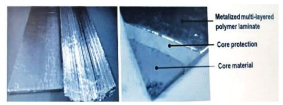
Figure 4: Vacuum insulation panels.
