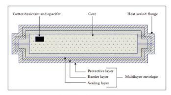
Fig.4. Schematic of a VIP Figure 6: Schematic of VIP.
