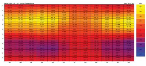
Figure 21: Rate of heat transfer through the envelope of model having aerogel panels over wall.
