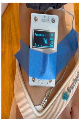
Figure 2: Pressure sensor with switch, Comparison of traditional straight edge strap and Rolled inner seam strap.
