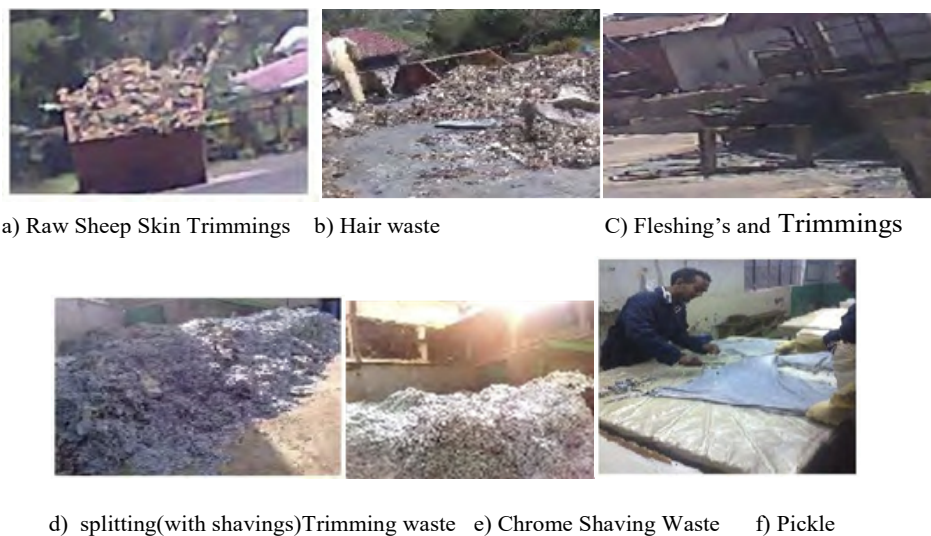
Figure 2: Generated of sludge and other solid wastes, pictured from Mojo Tannery Share company, Ethiopia.
