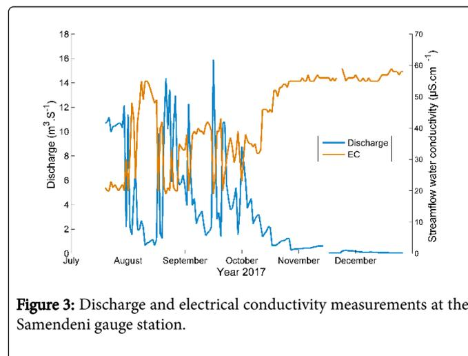
**Figure 3:** Discharge and electrical conductivity measurements at the Samendeni gage station.
