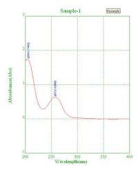
Figure 3: UV Spectrum of carbimazole.
