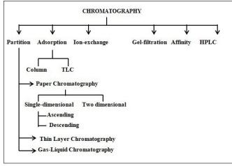
Figure 1: Classification of chromatographic methods.
