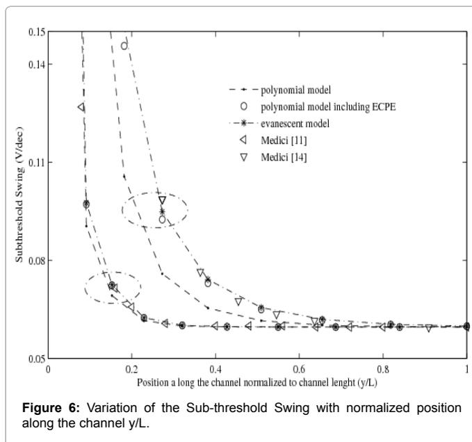
Figure 6: Variation of the Sub-threshold Swing with normalized position along the channel y/L.
