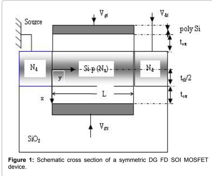
Figure 1: Schematic cross section of a symmetric DG FD SOI MOSFET device.
