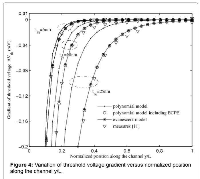
Figure 4 illustrates the evolution of the threshold voltage gradient in regard to the normalized position to  $L$  along the channel for  $L=150nm$ ,  $V_{ds}=1.5V$ ,  $t_{ox}=1.5nm$  and for  $t_{Si}=5, 10$  and  $25nm$ . These results prove a perfect agreement, at  $d_{eff}=0.25t_{si}$ , between the evanescent model and the polynomial model including the ECPE with Jaju's measurements [11].
