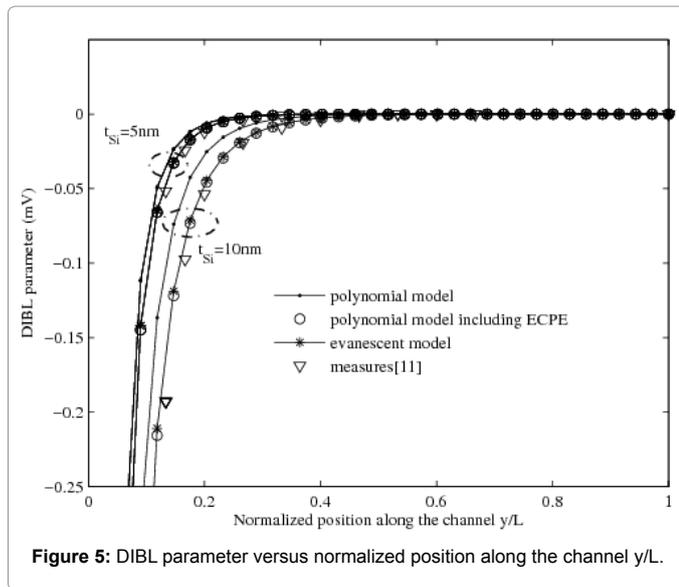
Figure 5: DIBL parameter versus normalized position along the channel y/L.
