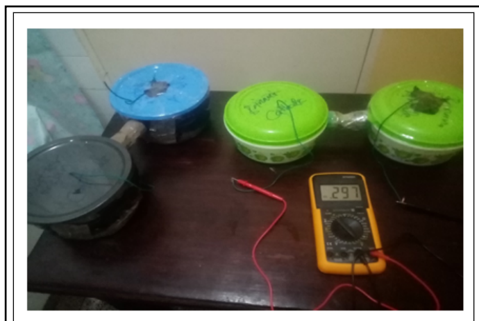
Figure 2: Fabricated microbial fuel cells chambers (composites).
