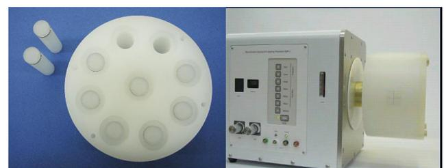
Figure 1: The standard phantom and test tubes.
