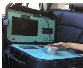
(b) PEMS installed in Backseat
