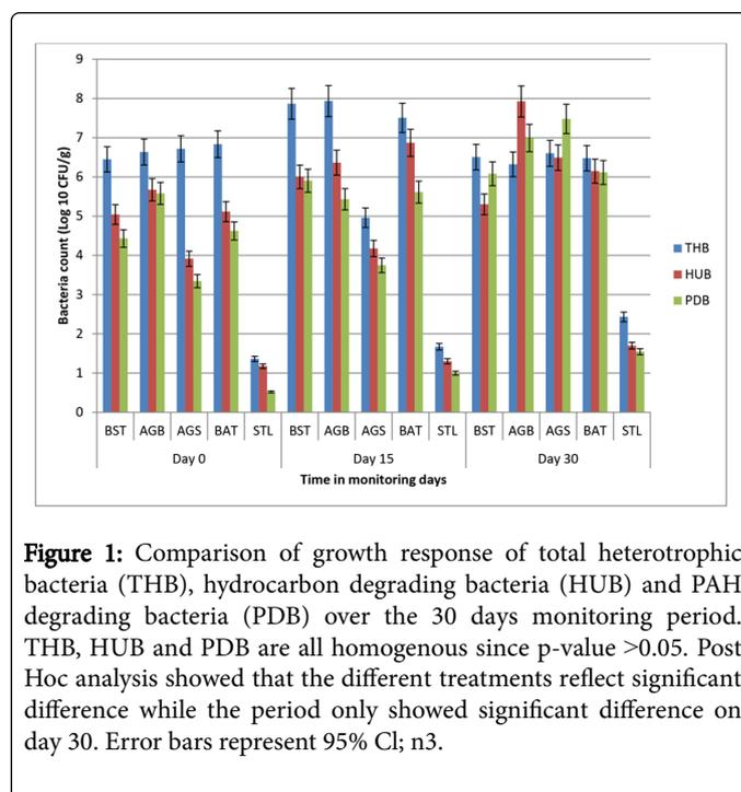
**Figure 1:** Comparison of growth response of total heterotrophic bacteria (THB), hydrocarbon degrading bacteria (HUB) and PAH degrading bacteria (PDB) over the 30 days monitoring period. THB, HUB and PDB are all homogenous since p-value >0.05. Post Hoc analysis showed that the different treatments reflect significant difference while the period only showed significant difference on day 30. Error bars represent 95% CI; n3.
