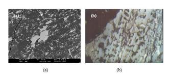
Figure 2: Backscattering image and optical microscope images of Inner Mongolian coal.
