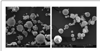
Figure 3: Morphology and microstructure of Inner Mongolian coal fly ash.
