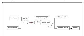
**Figure 7:** Typical Acid Alkaline combined method diagram.
