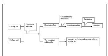
Figure 6: Typical acid-soluble ash treatment process diagram.
