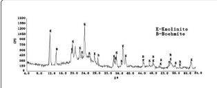
Figure 1: XRD analysis of Inner Mongolian coal.
