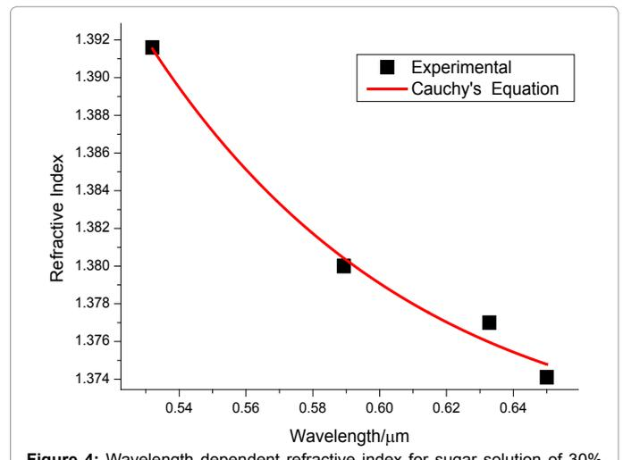
Figure 4: Wavelength dependent refractive index for sugar solution of 30% at room temperature a. the dot indicate experimental results and b. the line indicate Cauchy's Equation.
