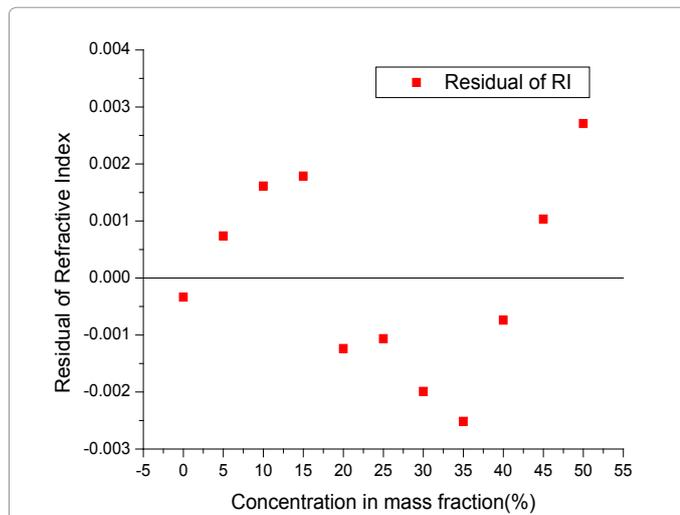
Figure 3: shows Residual of RI of sugar solution at room temperature.
