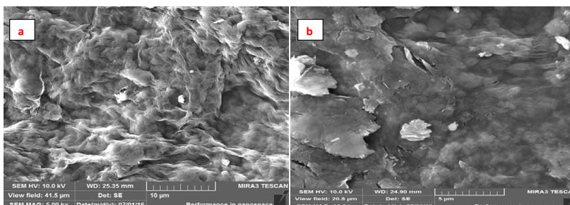
Figure 4: (a, b) Scanning electron microscopy image of GO 10 µm resolution and RGO at 5 µm resolution.
