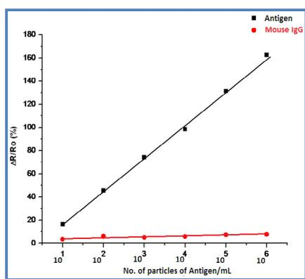
Figure 6c: Depicts the increase in resistance with the higher concentration of antigen while the non-specific Mouse IgG shows the low specificity with the FET.
