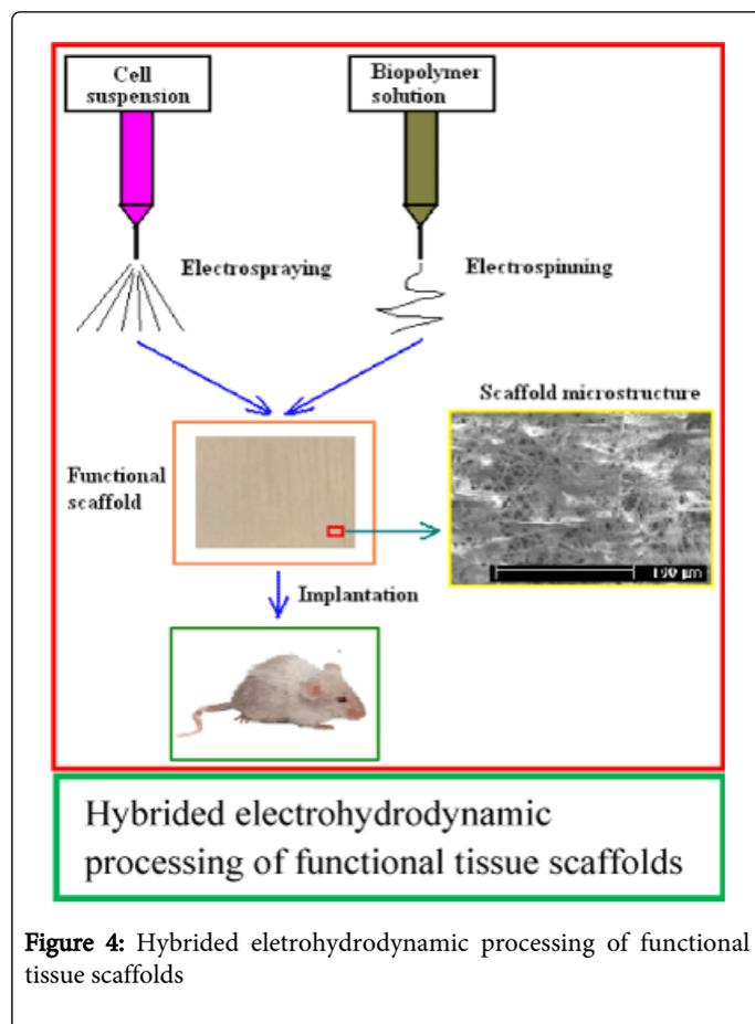
**Figure 4:** Hybrid electrohydrodynamic processing of functional tissue scaffolds
