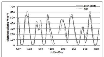
**Figure 8:** Variation between observed (solid line) shortwave radiation during BOBMEX (Bay of Bengal Monsoon Experiement) and calculated shortwave radiation (dotted line) with the new formulae.
