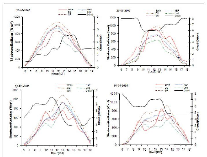
Figure 6: Variations of observed and calculated incoming shortwave radiation using different methods (SWin – Observed shortwave radiation, calculated shortwave radiation from the different formulae NEF – formulae developed by the authors, Lind - from the Lind [17], GR- Gopala Reddy [18] and DS - Dobson and Smith [15] and Cloud – cloud amount.
