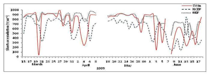
Figure 7a: Variations of Observed shortwave radiation (thick line), shortwave radiation from the NCEP (dashed line) and calculated incoming shortwave radiation with New Empirical Formulae (NEF) (dotted line) during March- June 2003 at 1130 IST.
