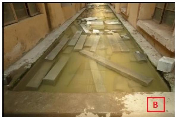
**Figure 3(B):** Photograph showing the casted specimens in the curing tank.
