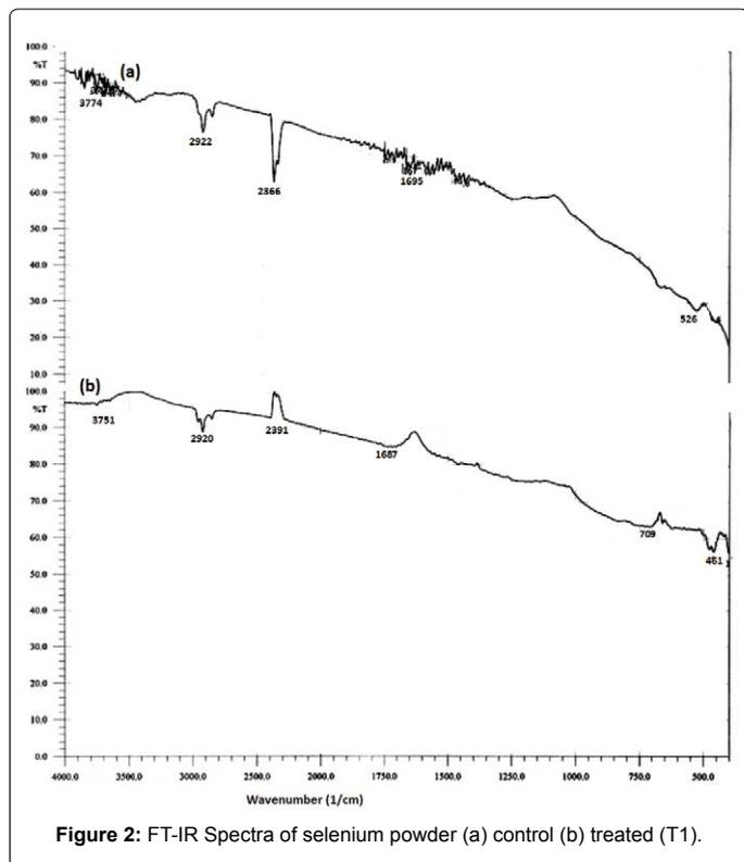
Figure 2: FT-IR Spectra of selenium powder (a) control (b) treated (T1).
