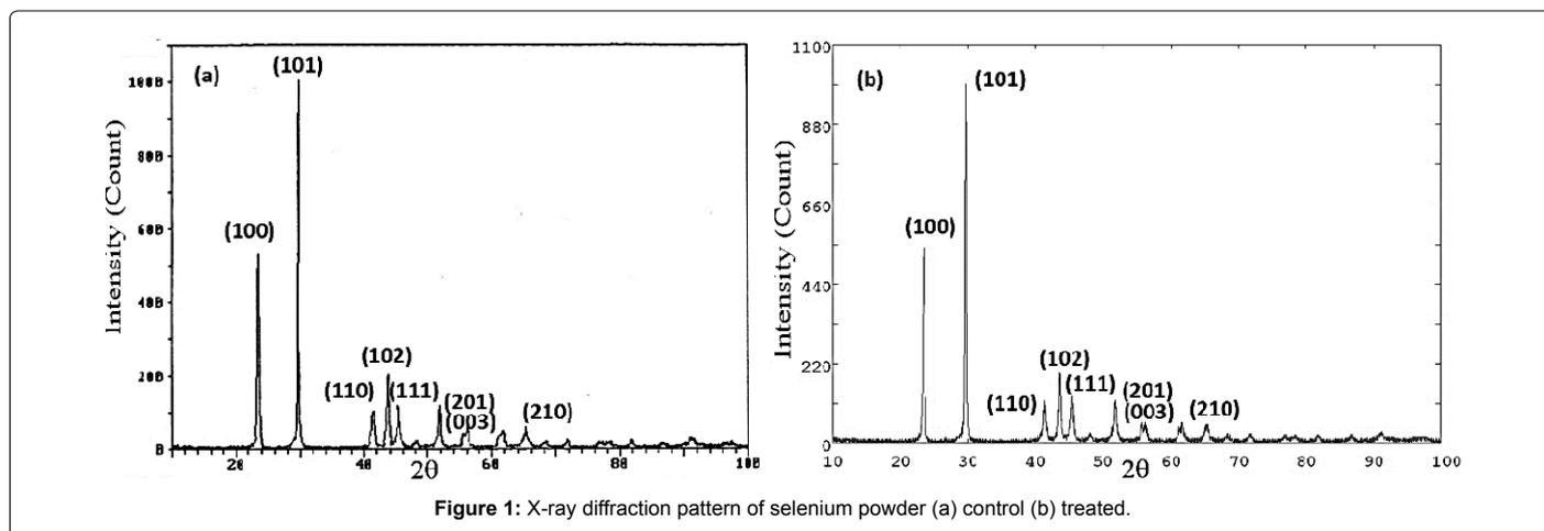
Figure 1: X-ray diffraction pattern of selenium powder (a) control (b) treated.
