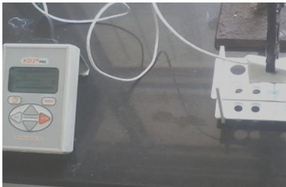
Figure 4: Shows the conductivity meter (KD2 PRO).
