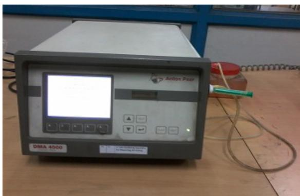
Figure 5: Shows density meter (Anton Paar-DMA 4500).
