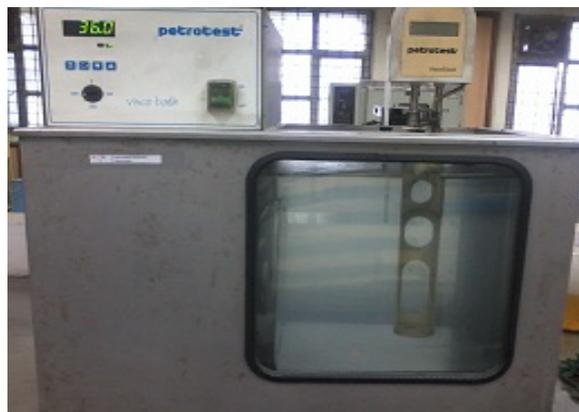
Figure 6: Shows the kinematic viscometer (Petrotest Viscobath).
