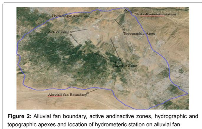
Figure 2: Alluvial fan boundary, active and inactive zones, hydrographic and topographic apexes and location of hydrometric station on alluvial fan.
