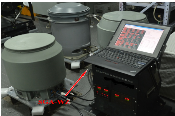
Figure 1: The SGA-WZ installed in the aircraft.
