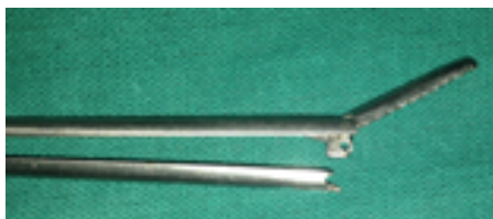
Figure 2: Metallic forceps with a fractured prong.
