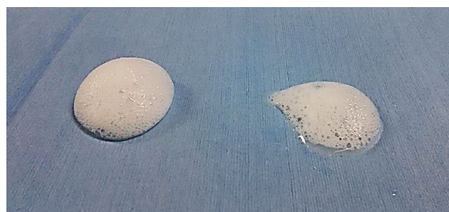
Figure 4: The foam began disappearing immediately even when a small amount of ethyl alcohol was sprayed on the foam cleanser detergent, completely disappearing in about 10 s.
