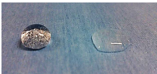
Figure 3: 200 µl of distilled water was dropped on a waterproof surgical cloth to form a sphere, and when a small amount of ethyl alcohol was dropped onto it, the sphere immediately flattened and the surface tension decreased.
