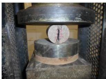
Figure 6: Loading set up and specimen for Brazilian test.
