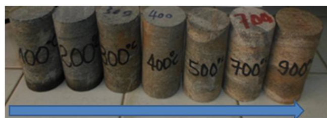
Figure 2: Visual degradation of samples during heating process.
