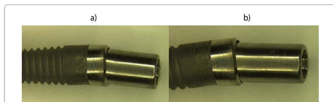
**Figure 9:** Failure mode of the Integrity Tapered Implants 2 pieces implant-abutment connection system. The failure mode of the Integrity Tapered Implants 1 and 2 piece abutment connection was an identical combined bending of the implant-abutment Connection.
