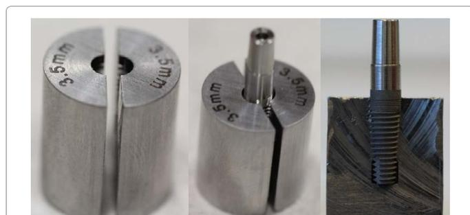
**Figure 2:** Custom made sleeves. Set of two metal sleeves (A-2 tool steel) to allow homogenous load distribution to the implant body.
