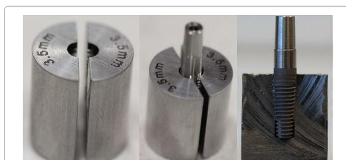
**Figure 2:** Custom made sleeves. Set of two metal sleeves (A-2 tool steel) to allow homogenous load distribution to the implant body.
