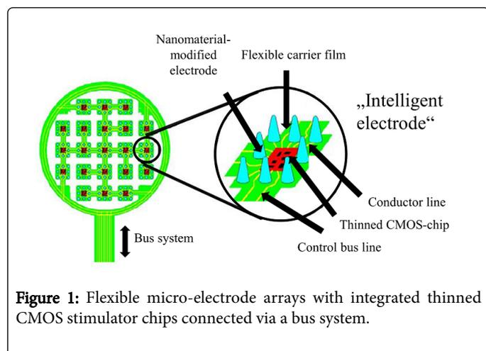
**Figure 1:** Flexible micro-electrode arrays with integrated thinned CMOS stimulator chips connected via a bus system.
