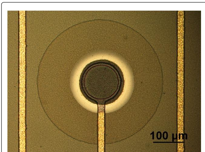
**Figure 10:** Flex-MEA: Pt/CNT electrode without bubble formation.
