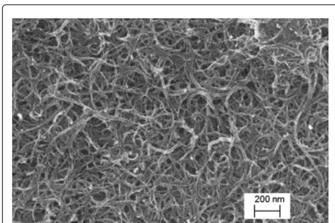
**Figure 11:** SEM image of Pt/CNT-electrode after EPD without bubble formation. (Image was taken by IHT, RWTH Aachen University)
