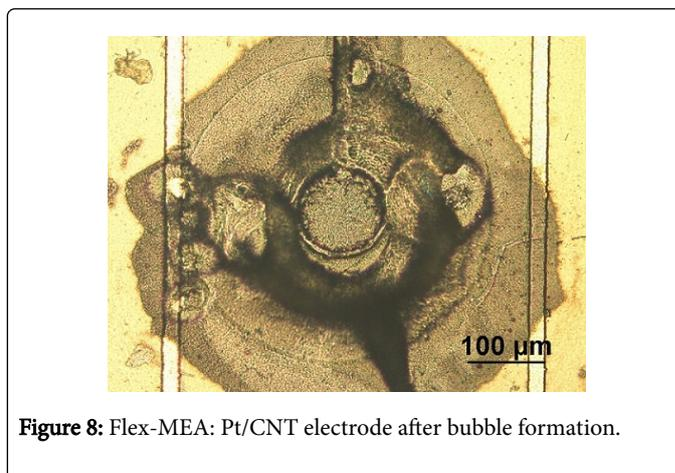
Figure 8: Flex-MEA: Pt/CNT electrode after bubble formation.
