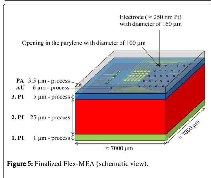
**Figure 5:** Finalized Flex-MEA (schematic view).
