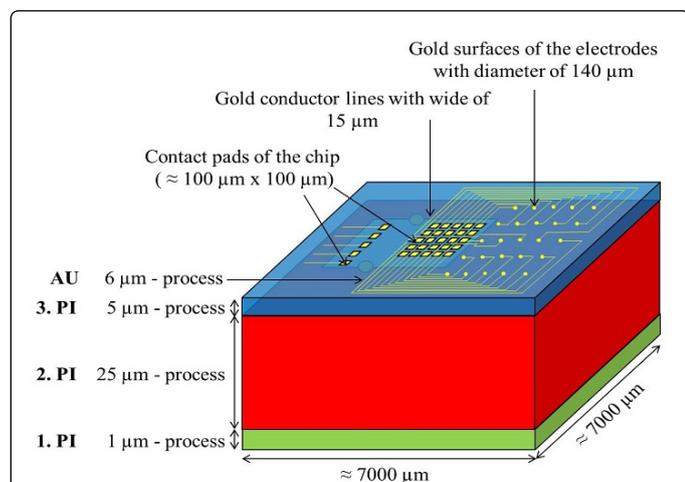
**Figure 4:** Contacting the CMOS stimulator chip to the gold surfaces of the electrodes.
