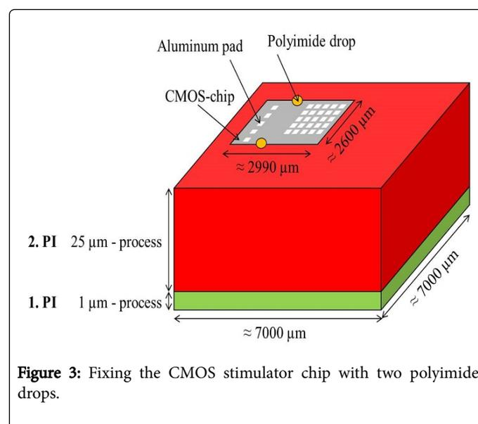
**Figure 3:** Fixing the CMOS stimulator chip with two polyimide drops.
