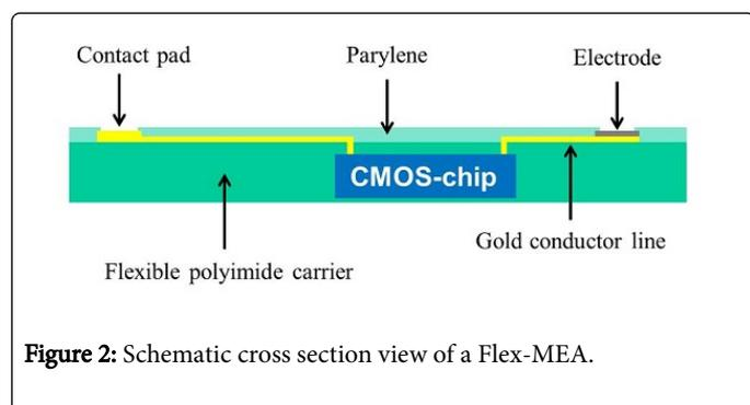
**Figure 2:** Schematic cross section view of a Flex-MEA.
