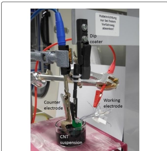
Figure 6: Measuring arrangement for the EPD.
