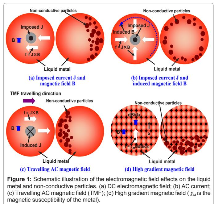
Figure 1: Schematic illustration of the electromagnetic field effects on the liquid metal and non-conductive particles. (a) DC electromagnetic field; (b) AC current; (c) Travelling AC magnetic field (TMF); (d) High gradient magnetic field ( $\chi_m$  is the magnetic susceptibility of the metal).
