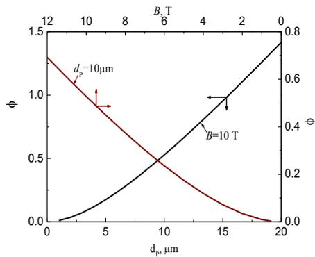
**Figure 2:** Effect of the particle size and magnetic flux density on the energy coefficient ( $\phi$ ). The calculation is based on alumina particles in liquid aluminum and the data needed for the calculation are taken from [30].
