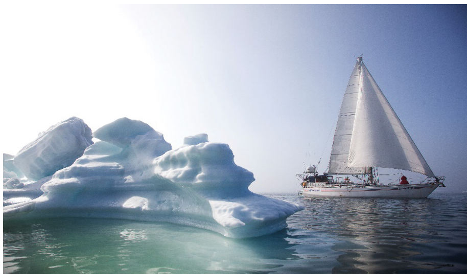
Figure 1: The legendary Northwest Passage: Length 15.17 m, 17.00 m with the aft bridge, and 4.34 m width. With a lift keel, the draft varies from 1.40 m and 2.90 m.
