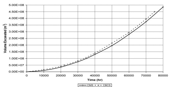
Figure 6: Volume of Circular Pit vs. Time using CMS and CycEx CBCS.
