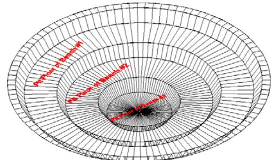
Figure 3: 3D View of a Circular Pit with 3 Benches.
