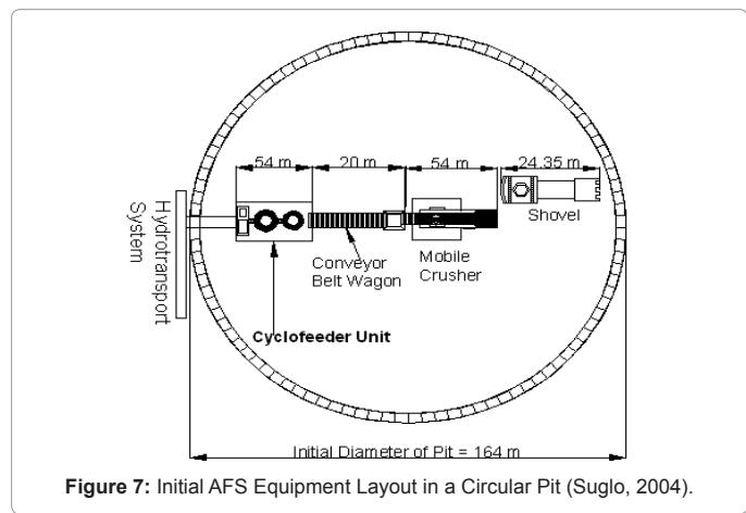
Figure 7: Initial AFS Equipment Layout in a Circular Pit (Suglo, 2004).
