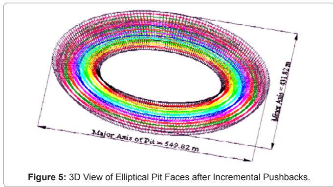
Figure 5: 3D View of Elliptical Pit Faces after Incremental Pushbacks.
