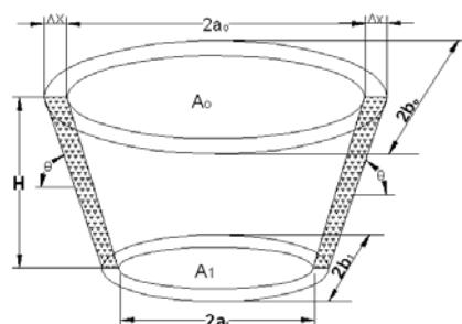
Figure 2: Elliptical Pit Section with one Incremental Pushback,  $\Delta x$ .
