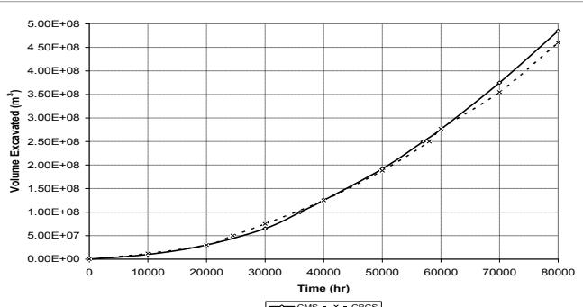
**Figure 8:** Elliptical Pit vs. Time using PDEs on Bench #1 for CMS and CycEx CBCS Option.
