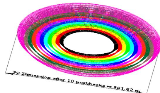
Figure 4: 3D Circular Pit Faces after taking Incremental Pushbacks on Bench #1.
