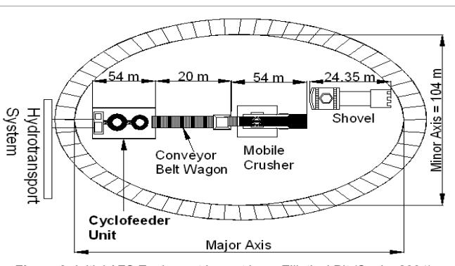
**Figure 9:** Initial AFS Equipment Layout in an Elliptical Pit (Suglo, 2004).
