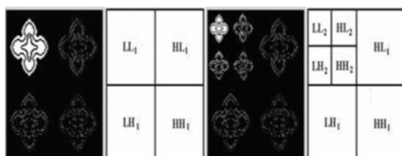
Fig.3 Results of the wavelet transformation analysis derived from various layers of a given image (a) 1-Level DWT image (b) 1-Level DWT Resolution (c) 2-Level DWT image (d) 2-Level DWT Resolution
