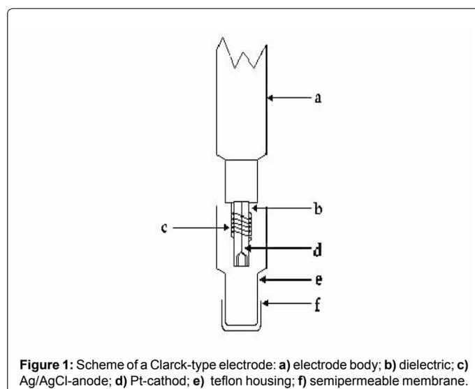
**Figure 1:** Scheme of a Clark-type electrode: a) electrode body; b) dielectric; c) Ag/AgCl-anode; d) Pt-cathode; e) teflon housing; f) semipermeable membrane.
