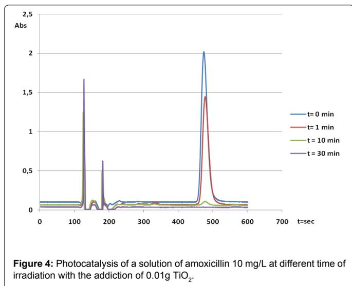
Figure 4: Photocatalysis of a solution of amoxicillin 10 mg/L at different time of irradiation with the addition of 0.01g TiO<sub>2</sub>.
