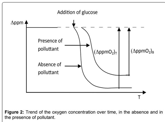
Figure 2: Trend of the oxygen concentration over time, in the absence and in the presence of pollutant.
