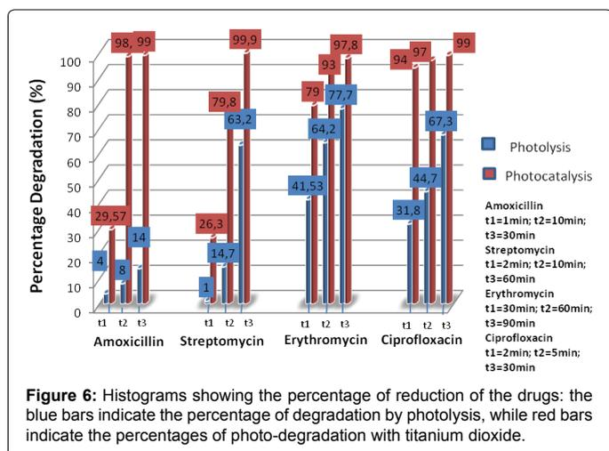
**Figure 6:** Histograms showing the percentage of reduction of the drugs: the blue bars indicate the percentage of degradation by photolysis, while red bars indicate the percentages of photo-degradation with titanium dioxide.
