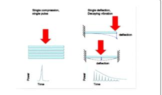
**Figure 5:** Difference in performance characteristics of single compression based and cantilever harvesters.
