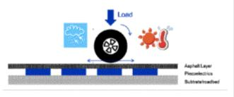
Figure 3: Piezoelectric road cross-section.
