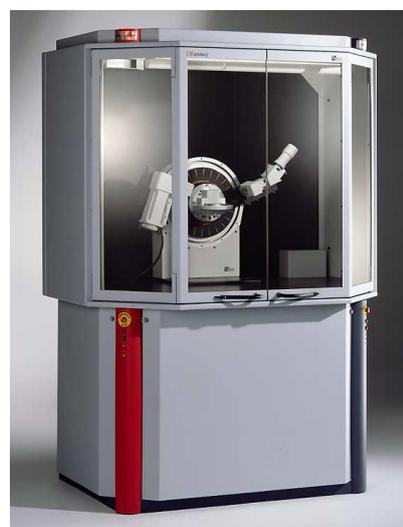
**Figure 1:** A PXRD (Bruker D8 Advance) showing the goniometer and its drives inside the cabinet.
