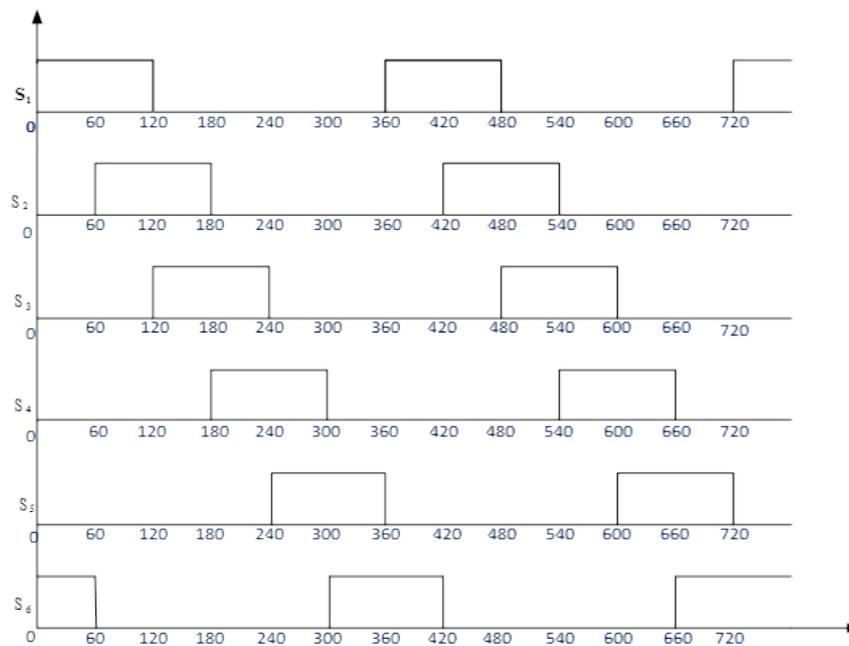
Figure 5: Waveform at 120° conduction for the Thyristors.
