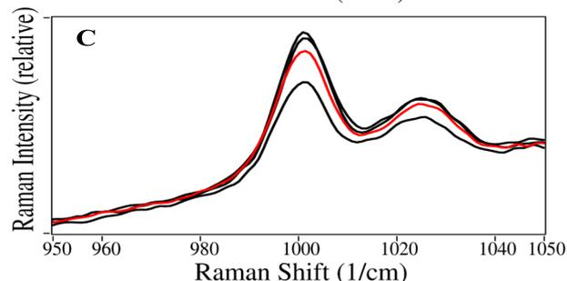
**Figure 6:** Representative SERS spectra of 100 ng/mL cocaine extracted from saliva. a) Capillary 1, position 10 (10-second spectrum), b) SERS of all 10 spots on capillary 1, c) SERS of the average spectra for all 4 capillaries; the red spectrum is the “unknown” sample.
