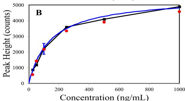
**Figure 7:** a) SERS of concentrated cocaine extracted from saliva containing 25, 50, 100, 250, 500, and 1000 ng/mL. Spectra are scaled to have the same background intensity. b) Plot of 1002 cm<sup>-1</sup> peak heights for each concentration (black squares connected by black line for clarity), Langmuir fit to data (blue line), and results for the 4th capillaries as unknowns (red dots). The standard deviation for the 100 ng/mL “unknown” sample is included.
