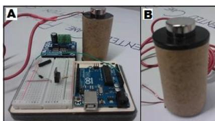
Figure 6: (A) Pulsing magnet apparatus and; (B) electromagnet coil.
