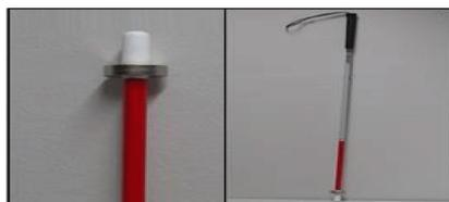
Figure 3: Augmented guidance cane.
