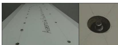
Figure 4: Magnet points trail test bed and pulsing magnet apparatus on it.
