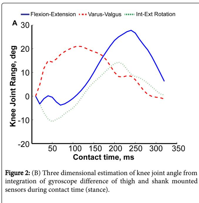
Figure 2: (B) Three dimensional estimation of knee joint angle from integration of gyroscope difference of thigh and shank mounted sensors during contact time (stance).
