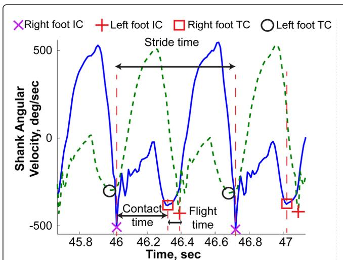
Figure 2: (A) Shank derived gyroscope data illustrating stride time, contact time and flight time.
