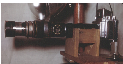
Figure 1B: Two early Japanese colposcopes used in colpophoto: 1960s Maeda, using Hektor 135 mm F4.5 Leica lens.
