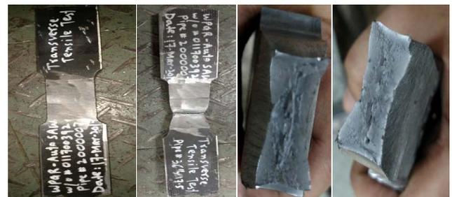
**Figure 1:** (Sequence of Picture Left to right): Prepared marked tensile specimen, fractured tensile specimen, fractured tensile specimen cone appearance, fractured tensile specimen cup appearance.
