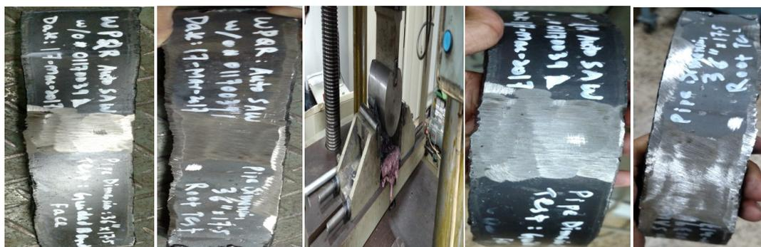
Figure 4: (Sequence of Picture Left to right): Prepared guided bend face specimen, guided bend root test specimen, guided bent test machine, face bent specimen showing no crack appearance, root bent specimen showing no crack appearance.
