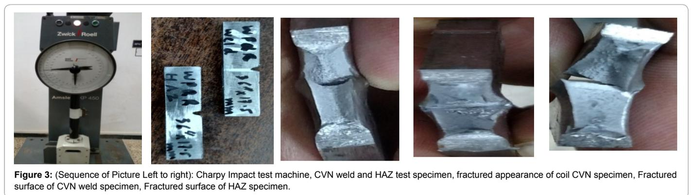
Figure 3: (Sequence of Picture Left to right): Charpy Impact test machine, CVN weld and HAZ test specimen, fractured appearance of coil CVN specimen, Fractured surface of CVN weld specimen, Fractured surface of HAZ specimen.
