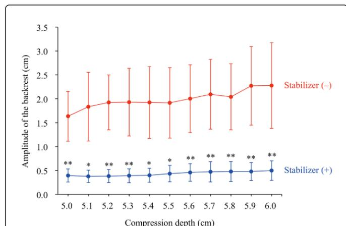
Figure 3: Effect of the stabilizer (round stool) on the vertical movements of the backrest caused by chest compressions. Results are expressed as mean ± standard deviation. Asterisks represent significant differences (\*P<0.05 and \*\*P<0.01).
