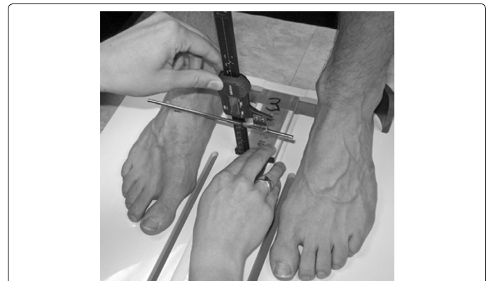
Figure 1: Digital gauge used to measure the dorsal arch height in weight bearing.
