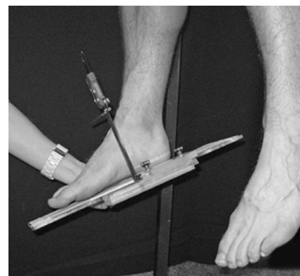
Figure 5: Placement of the portable platform under the plantar surface of the foot.
