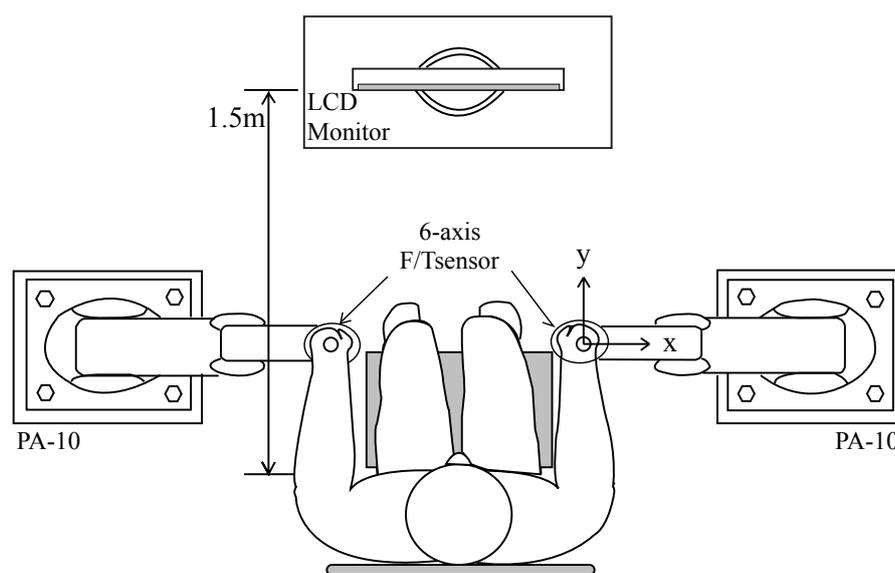
Figure 1: Top view of experimental setup.
