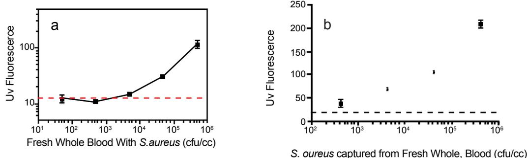
**Figure 7:** Comparison of the limit of detection using fluorescence measurements of the reduced pyridine nucleotides of *Staphylococcus aureus* in fresh whole blood (a) captured in a 0.2 mm thick quartz cell with that achieved on (b) a tethered-ligand quartz surface and rinsed to remove the blood. The dashed line is the uncontaminated fresh whole blood control.
