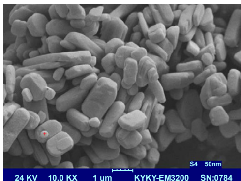
Figure 3: SEM image of nano nalidixic acid demonstrate amorphous morphology with a dimension of 50-60 nm.
